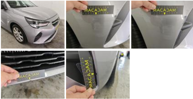
Bonnet, Stone chip(s), Repair and paint (complete)
