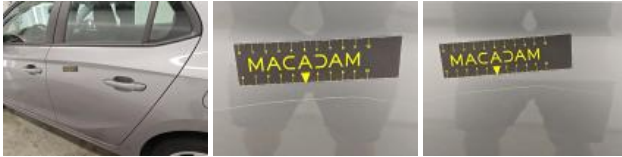
Wing RL, Dent(s), Repair and paint (complete)
