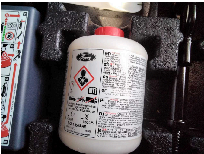
Damage 1: Equipment: Tirefit filler - Expired - Replace
