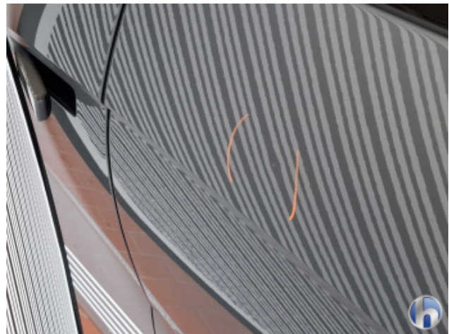
1. Tür Hinten - Links 1 Delle - Sanft Instandsetzen
