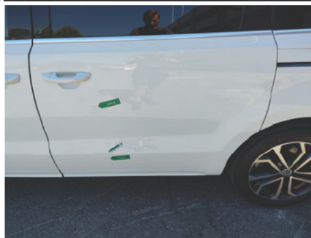
Tür / Hinten Links / Kratzer
