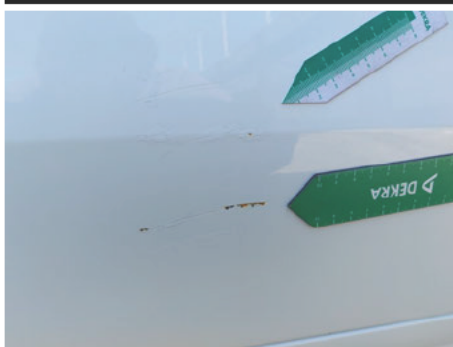
Tür / Hinten Links / Kratzer
