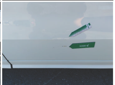
Tür / Hinten Links / Kratzer
