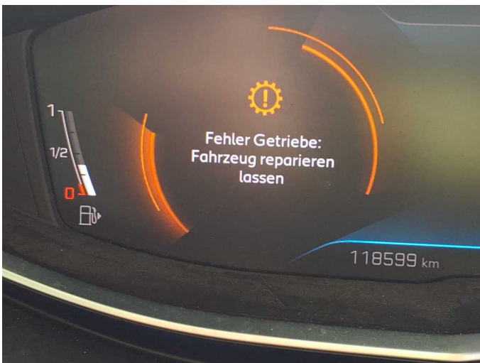
Damage 3: Gearbox: Gearbox - Non-operational - Perform diagnosis
