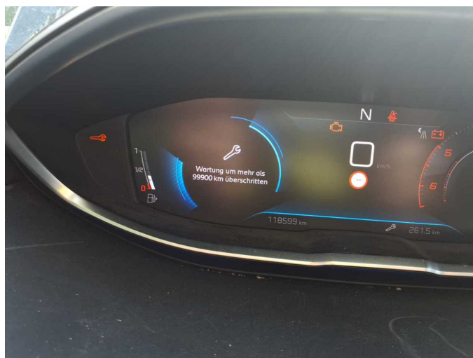
Damage 7: Misc.: Inspection / maintenance - Expired - Replace
