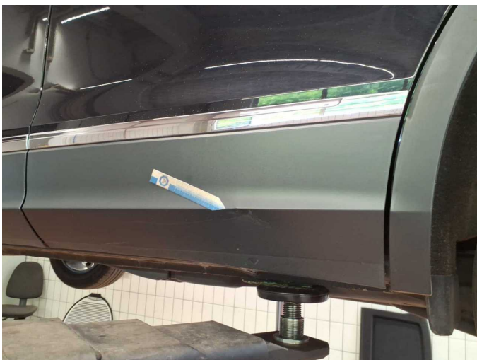
Damage 3: Door - rear left side: Brightware - lower - Deformed - Replace
