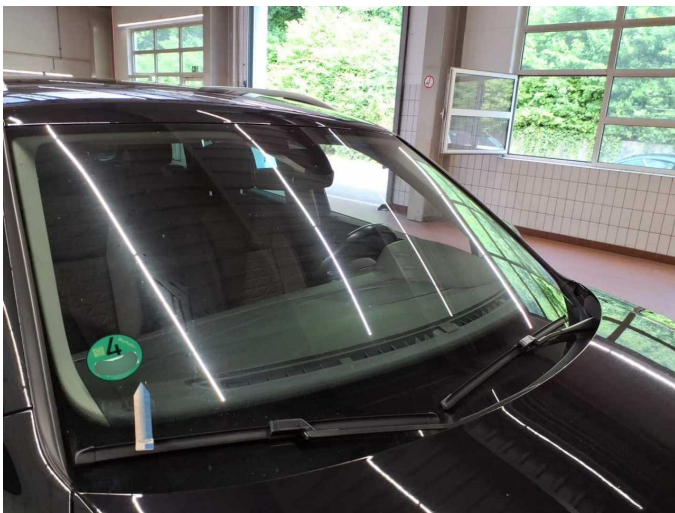
Damage 7: Vehicle glazing: Windscreen - Stone chips - Replace
