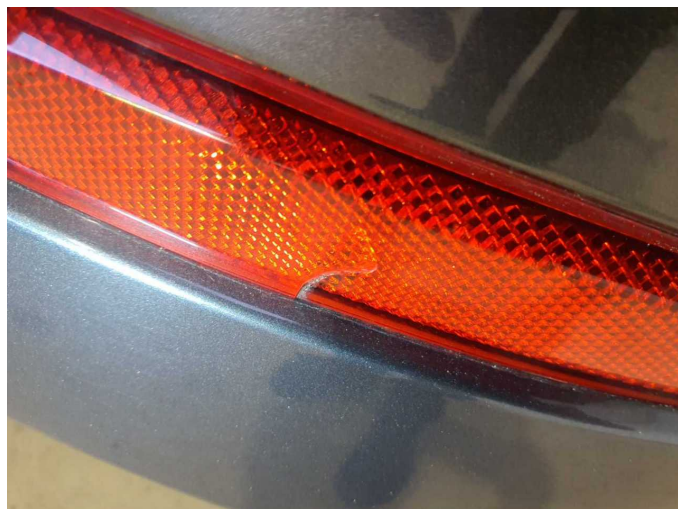
Damage 11: Boot lid / rear door: Reflectors - Broken / torn - Replace
