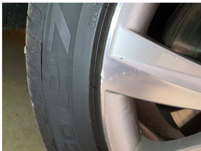
Damage 12: Wheel / tyres: Alloy rim - front right side - Scratch(es) - Loss in value
