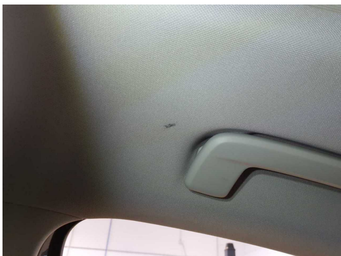
Damage 6: Trim / covers: Roof lining - Burn hole (cigarettes) - Smart repair
