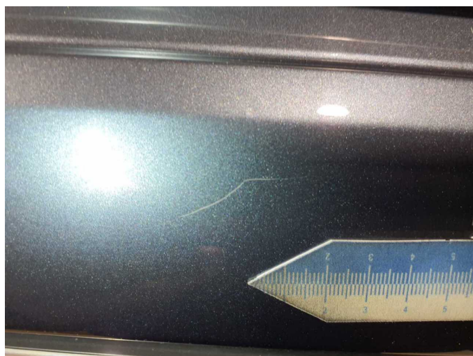
Damage 9: Roof: Roof rail - left side - Scratch(es) - Smart repair
