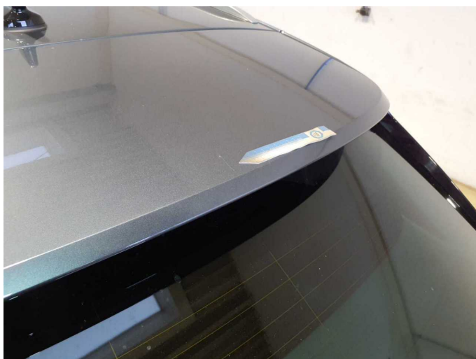
Damage 7: Boot lid / rear door: Rear spoiler - Scratch(es) - Smart repair
