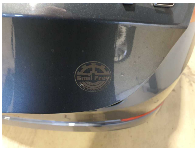
Damage 4: Boot lid / rear door: Boot lid - Glued / labelled - De-glue / neutralise
