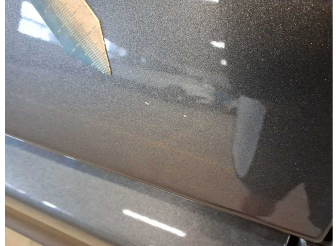
Damage 1: Door - front left side: Door - Stone chips - Smart repair
