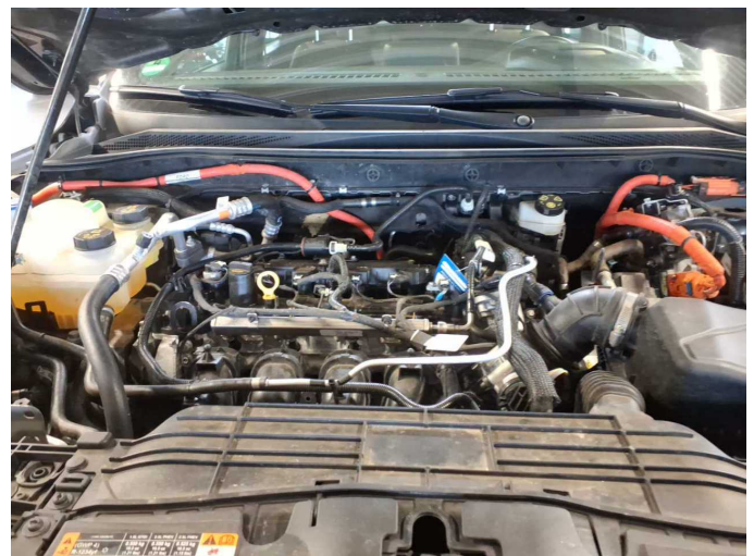
Missing part 1: Engine: Engine cover - Missing - Replace
