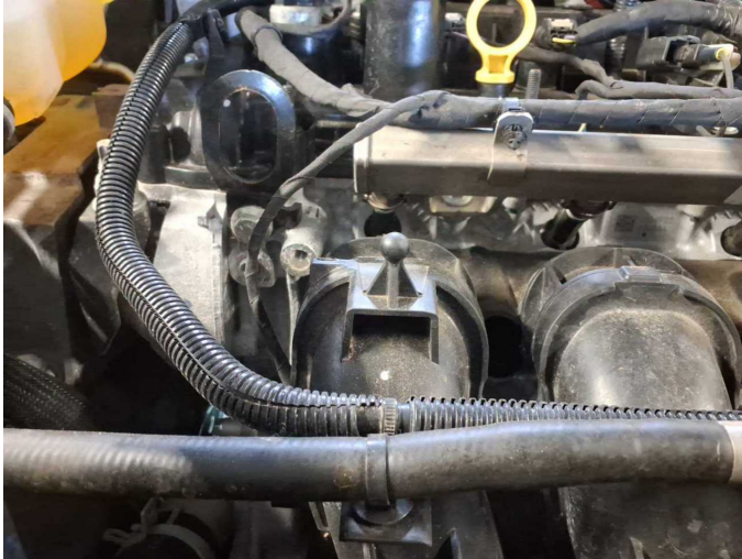
Missing part 1: Engine: Engine cover - Missing - Replace
