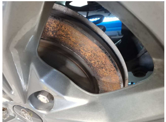
Damage 2: Braking system: Brake discs and pads - rear (Verschleißgrenze) - Corrosion - Replace
