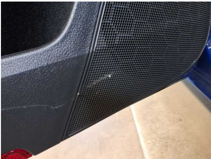
Damage 16: Trim / covers: Door trim - rear left side - Scratched - Loss in value
