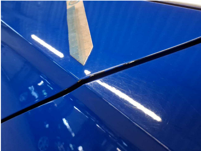
Damage 4: Door - rear left side: Door edge - Scratch(es) - Smart repair
