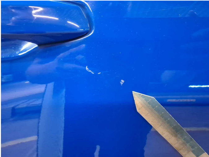
Damage 19: Door - rear right side: Door - Dent / paintcoat damage - Repair and paint
