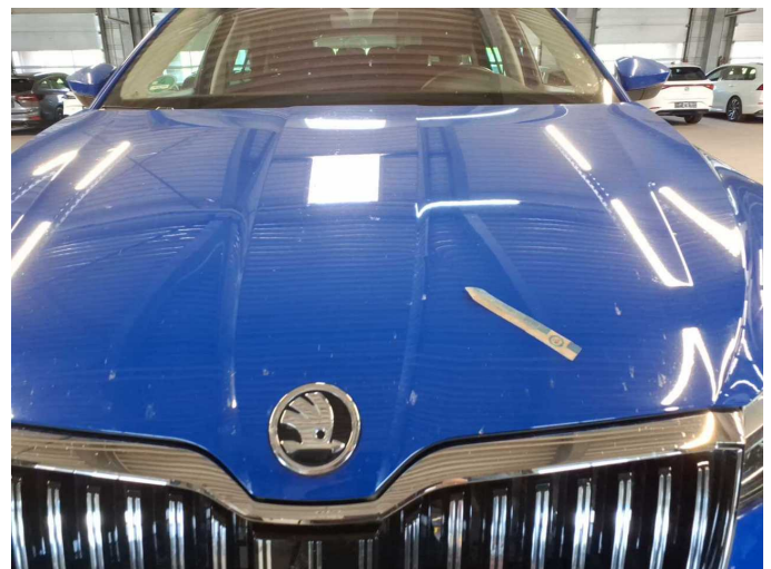
Damage 13: Bonnet: Bonnet - dent(s) - Smooth repair work
