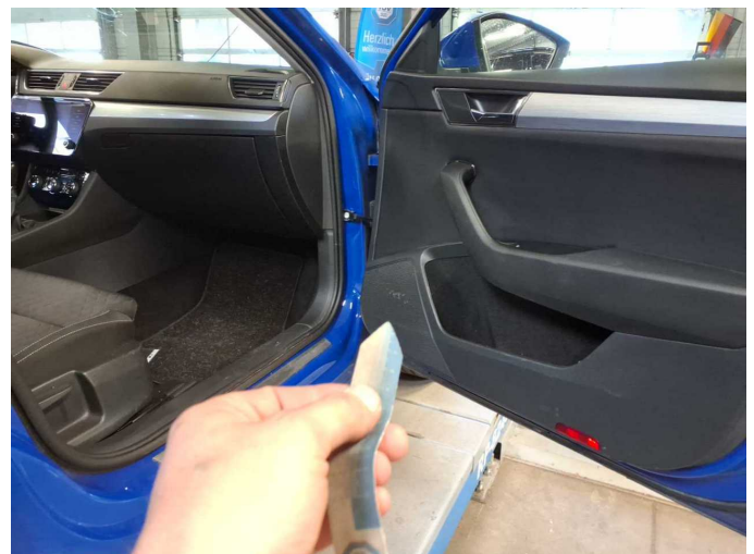
Damage 7: Door - front right side: Speaker cover - Scratched - Loss in value
