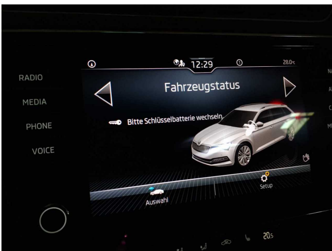
Damage 3: Equipment: Vehicle key (Batterie) - Empty - Replace
