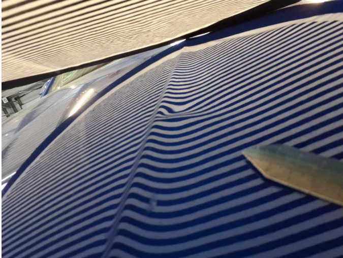
Damage 13: Bonnet: Bonnet - dent(s) - Smooth repair work
