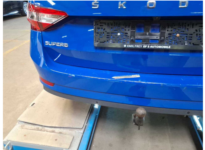
Damage 20: Rear bumper: Rear bumper - Scratched - Repair and paint
