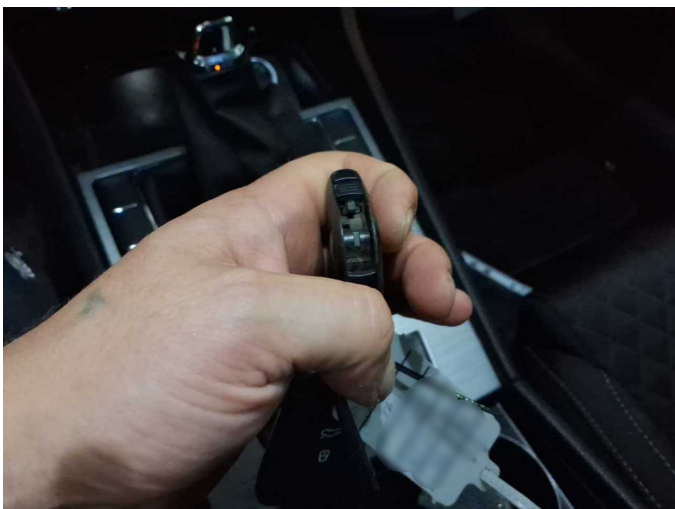
Damage 17: Equipment: Vehicle key with remote control (Schlüsselbart fehlt) - Incomplete - Replace
