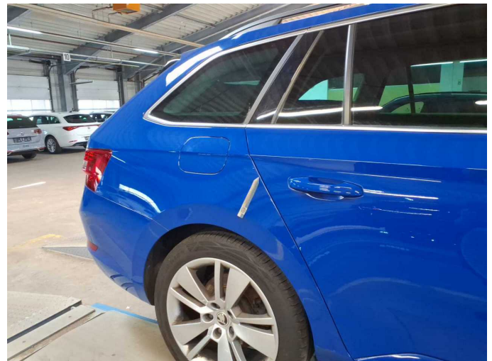
Damage 6: Side panel - rear right side: Side panel (Kante) - Scratch(es) - Smart repair
