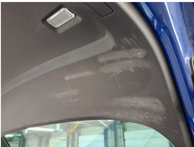
Damage 14: Trim / covers: Boot lid - interior trim - Scratched - Replace
