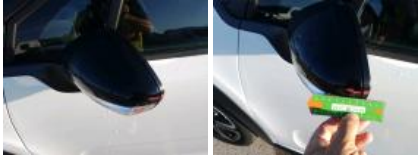
Outside rear-view mirror housing L, Scratch(es), Repair and paint (complete)
