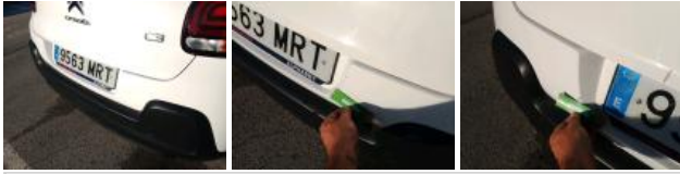
Bumper R, Scratch(es), Repair and paint (complete)
