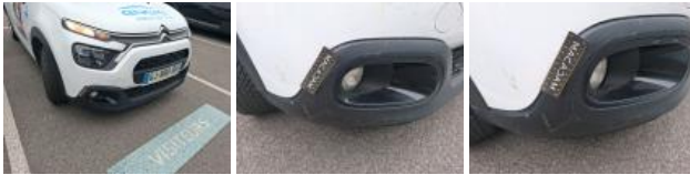
Bumper R, Broken, Replace
