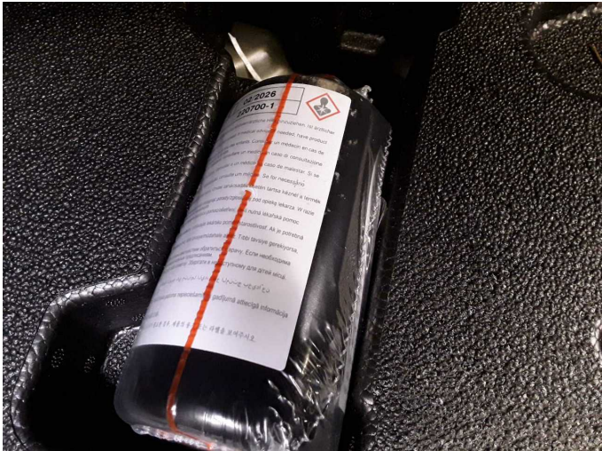
Damage 1: Equipment: Tirefit filler - Expired - Replace
