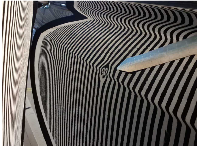
Damage 6: Door - front right side: Door - dent(s) - Smooth repair work
