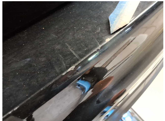
Damage 8: Rear bumper: Rear bumper - Scratched - Paint
