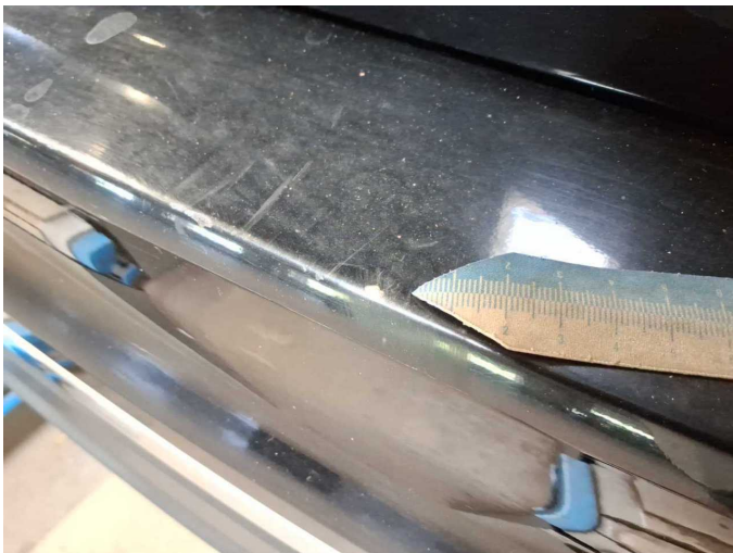
Damage 8: Rear bumper: Rear bumper - Scratched - Paint
