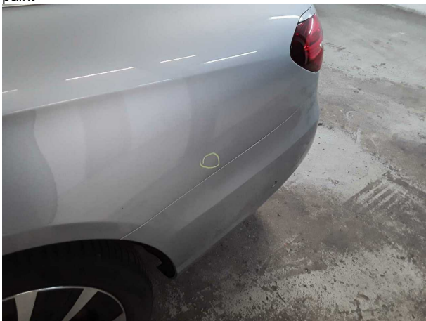
Damage #6: Side panel - rear left side: Side panel - Dent / paintcoat damage - Repair and paint
