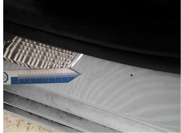
Damage #2: Sill - left side: Sill (vorne) - dent(s) - Smart repair
