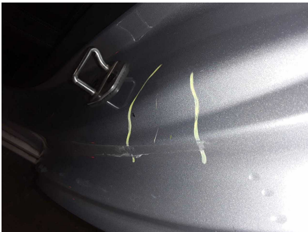
Damage #3: Side panel - rear left side: Sill - Scratched - Smart repair
