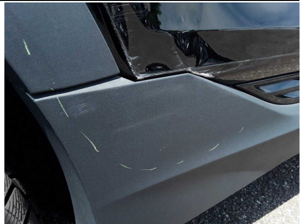
Damage #5: Door - rear right side: Brightware - lower - Scratched - Replace
