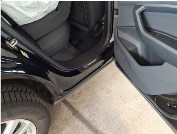
Damage #2: Trim / covers: Brightware / decorative strip - dent(s) - Replace
