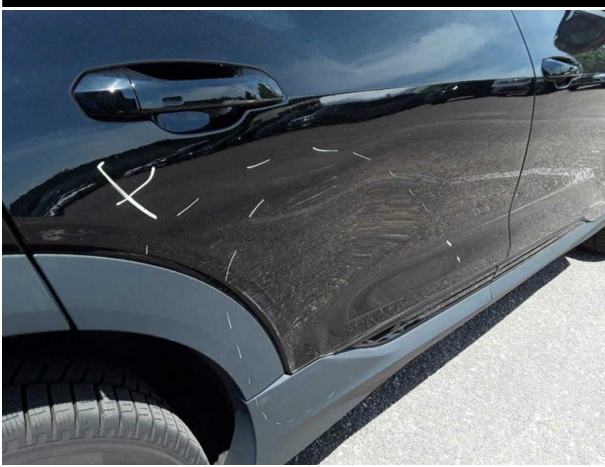
Damage #7: Door - rear right side: Door - Deformed - Replace
