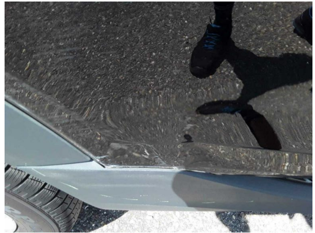
Damage #7: Door - rear right side: Door - Deformed - Replace
