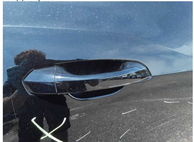
Damage #4: Door - rear right side: Door handle - outside - Scratched - Smart repair
