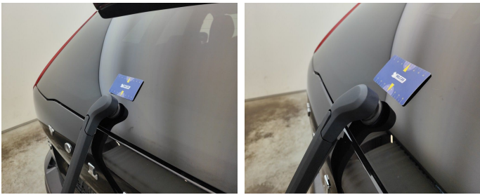
Back Side / Whiper Arm / Replace-cracked
