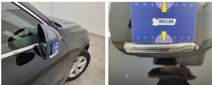
Side View Mirror Right / Direction Indicator / Replace-scratch
