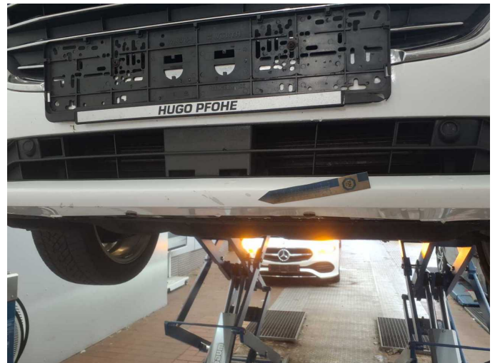
Damage 10: Front bumper: Front bumper - Scratch(es) - Paint
