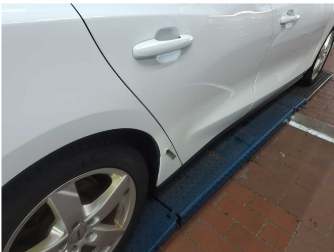
Wear and tear 9: Side panel - rear right side: Elbow - dent(s) - Smooth repair work
