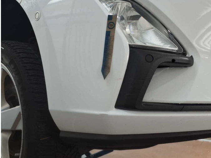
Damage 10: Front bumper: Front bumper - Scratch(es) - Paint
