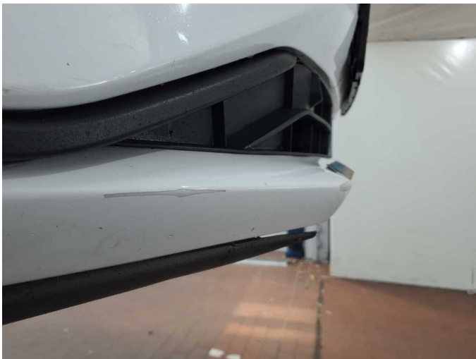
Damage 10: Front bumper: Front bumper - Scratch(es) - Paint
