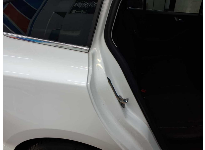
Wear and tear 8: Side panel - rear right side: Sill - Scratch(es) - Cover / polish
