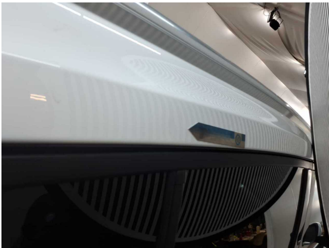
Wear and tear 6: Roof: Roof rail - right side - dent(s) - Smooth repair work
