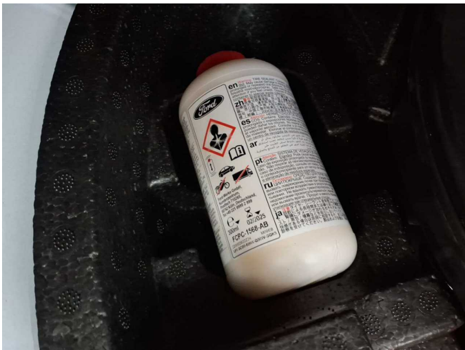
Damage 3: Equipment: Tirefit filler - Expired - Replace
