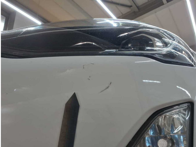
Damage 10: Front bumper: Front bumper - Scratch(es) - Paint
