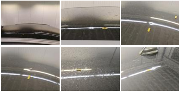
Roof, Hail damage, Paintless dent repair (hail)
