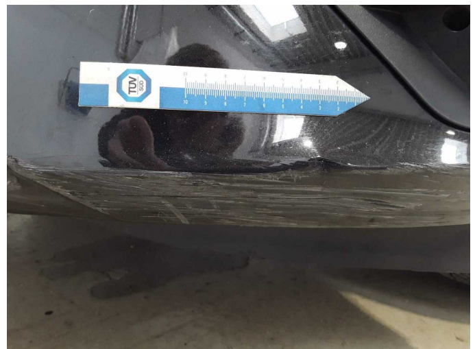
Damage 12: Front bumper: Front bumper - Dent / paintcoat damage - Replace
