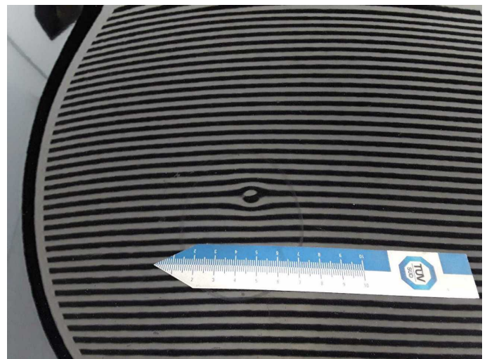
Damage 3: Bonnet: Bonnet - dent(s) - Smooth repair work
