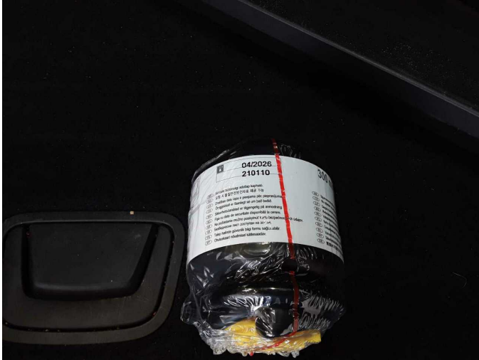
Damage 1: Equipment: Tirefit filler - Expired - Replace
