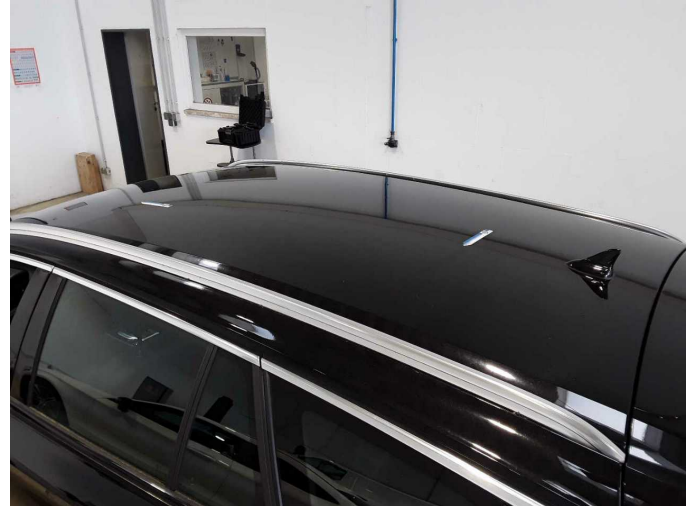
Damage 2: Roof: Roof - dent(s) - Smooth repair work
