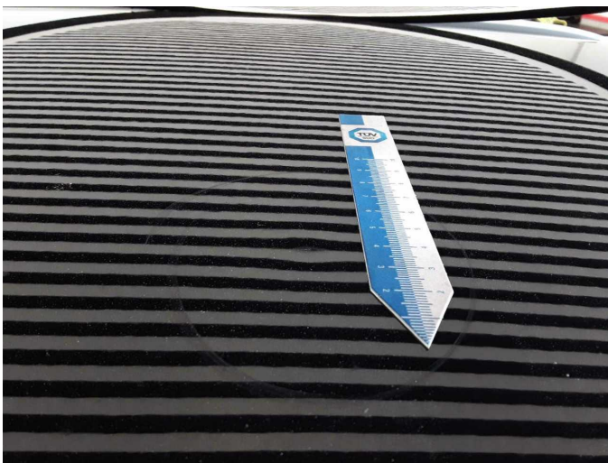
Damage 2: Roof: Roof - dent(s) - Smooth repair work
