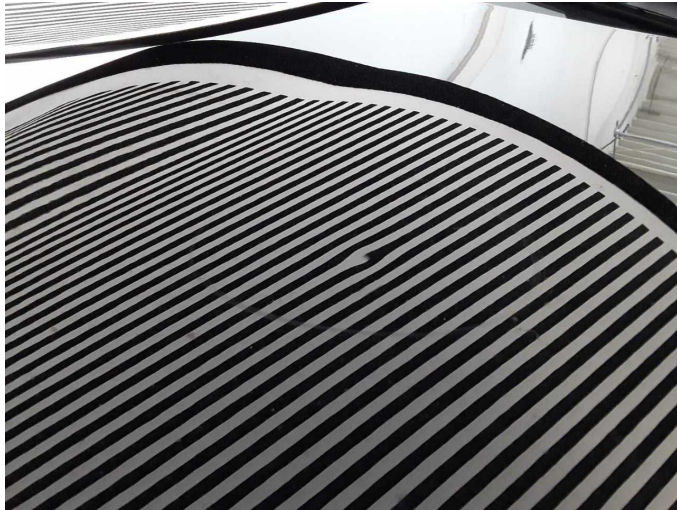
Damage 3: Bonnet: Bonnet - dent(s) - Smooth repair work
