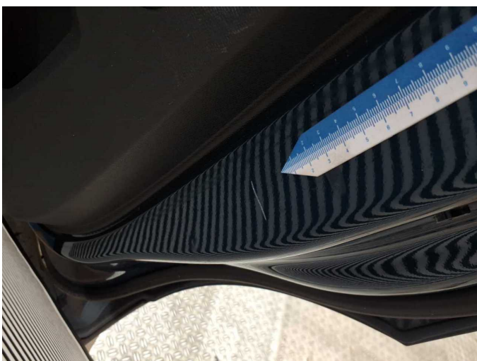
Damage 2: Door - rear right side: Door (Tür innen) - Dent / paintcoat damage - Repair and paint
