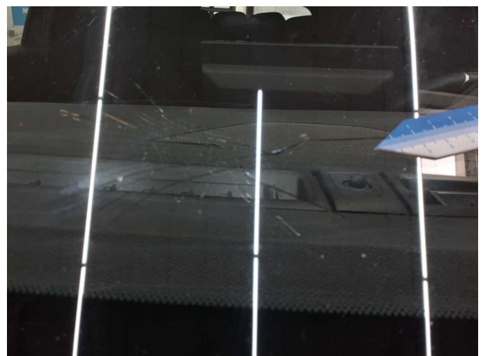
Damage 4: Vehicle glazing: Windscreen - Broken / torn - Replace
