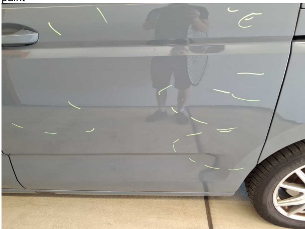
Damage #10: Sliding door - left side: Sliding door with glass pane... Scratched - Repair and paint
