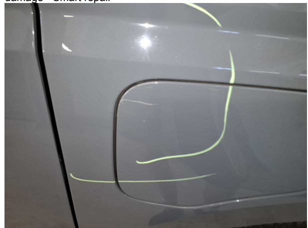
Damage #4: Fuel system: Tank cap - Scratched - Smart repair
