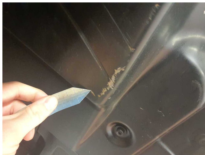
Damage 6: Body: Partition wall - Dent / paintcoat damage - Loss in value
