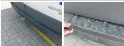
Outer sill R, Dent(s) and scratch(es), Repair and paint (complete)
