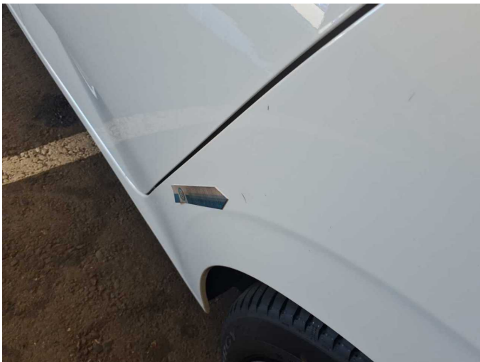
Damage 4: Side panel - rear left side: Side panel - Scratch(es) - Paint
