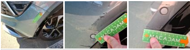
Door FR, Dent(s), Repair and paint (complete)
