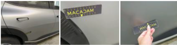
Door trim RR, Scratch(es), Replace and paint
