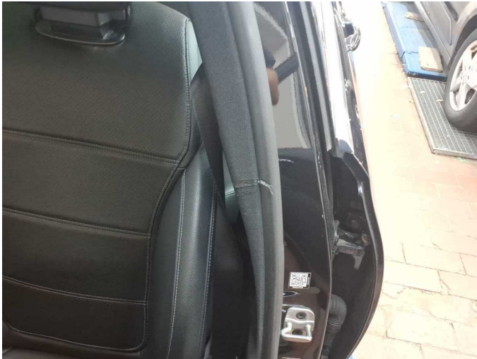
Damage 1: Trim / covers: A-pillar - trim - interior, left side - Scratch(es) - Replace
