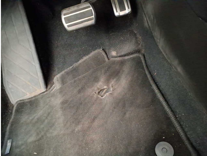
Damage 1: Trim / covers: Floor mats (Vorne links) - Damaged - Replace
