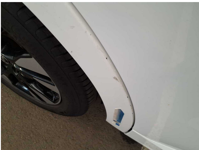
Damage 3: Side panel - rear right side: Wheel well extension - Scratch(es) - Smart repair
