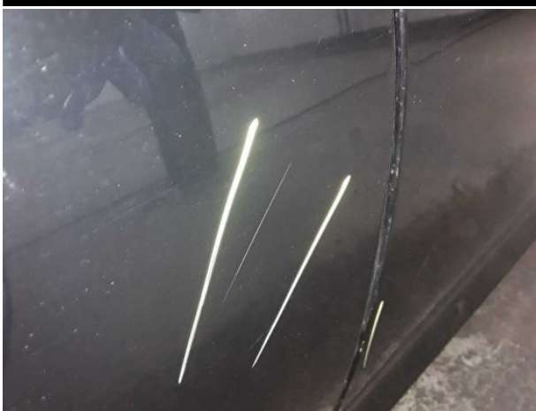
Damage #12: Door - rear right side: Door - Scratched - Repair and paint
