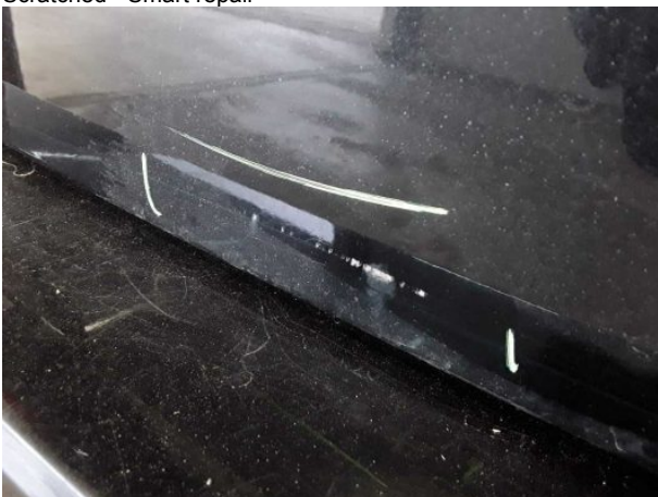
Damage #9: Boot lid / rear door: Boot lid - Scratched - Smart repair
