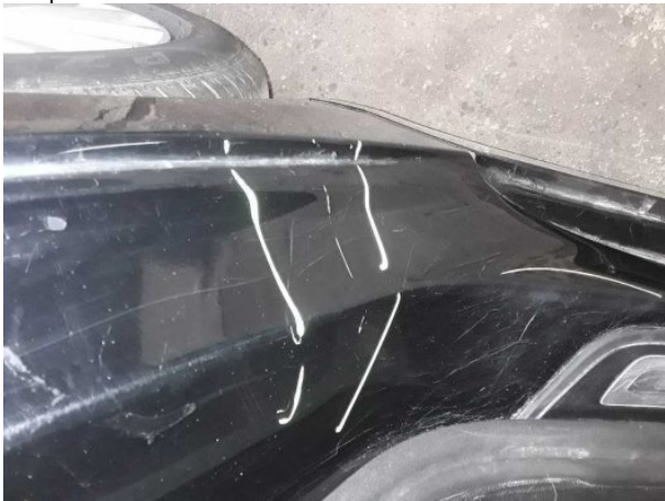
Damage #10: Side panel - rear left side: Sill - Scratched - Repair and paint
