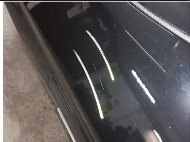
Damage #7: Mudguard - left side: Mudguard - left side - Scratched - Smart repair
