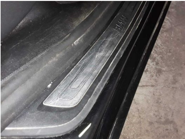
Damage #3: Side panel - rear right side: Sill (Leiste) - Scratched - Replace
