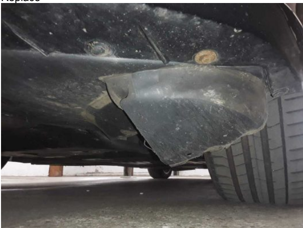
Damage #5: Body: Underbody panelling - Damaged - Replace
