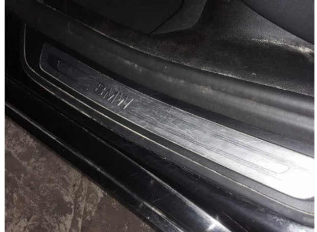
Damage #2: Side panel - rear left side: Sill (Leiste) - Scratched - Replace
