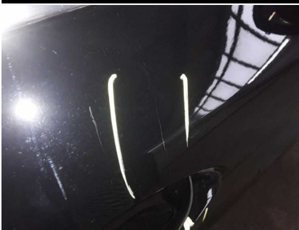
Damage #15: Door - front right side: Door - Scratched - Repair and paint
