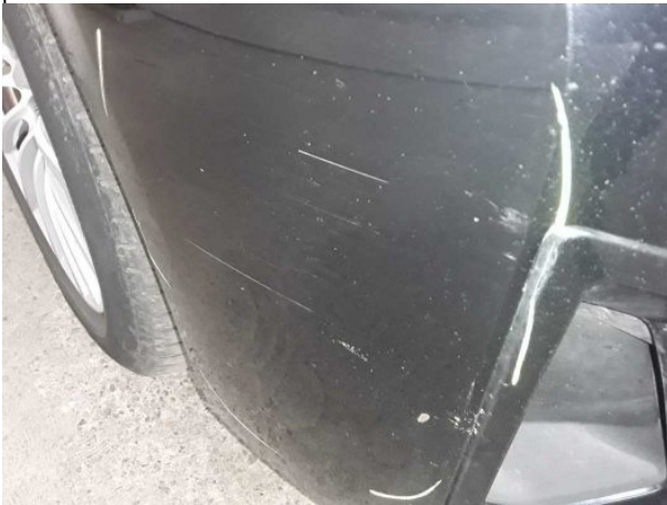
Damage #14: Front bumper: Front bumper - Scratched - Repair and paint
