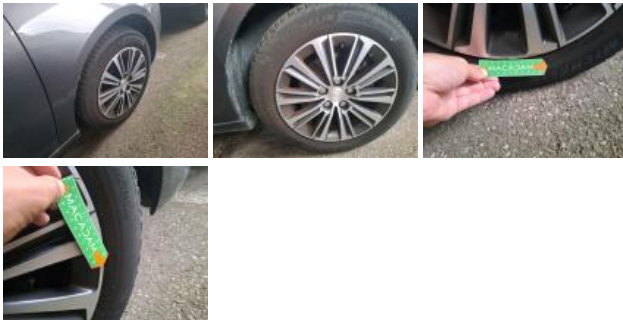
Tyre RR, Out of tolerance, Replace
