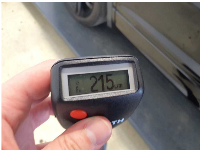
Repainting 3: Door - front left side
