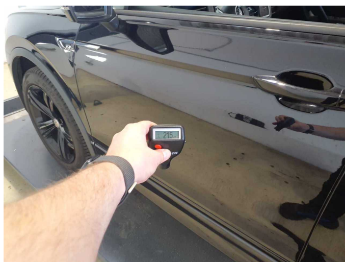
Repainting 3: Door - front left side
