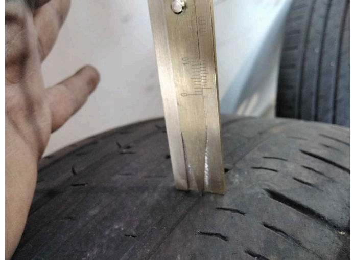
Damage 7: 2nd wheel set: 2 tyres (2mm) - Expired - Replace
