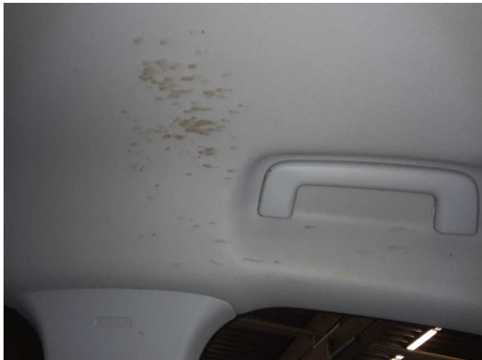
Damage 1: Trim / covers: Roof lining - Soiled - Clean
