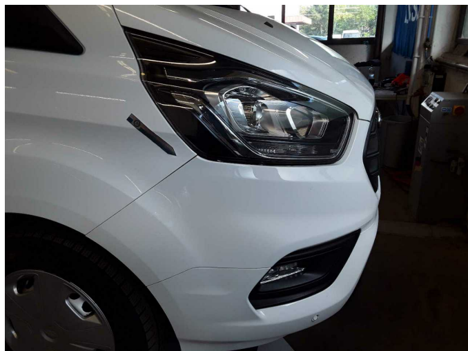
Damage 3: Front bumper: Front bumper - Malposition - Set / adjust
