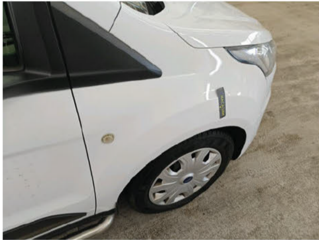
Wing FR Bad repair Repair and paint (complete) Right
