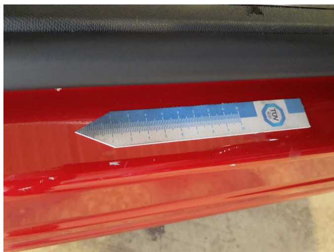
Damage 6: Sill - right side: Sill - Scratch(es) - Paint
