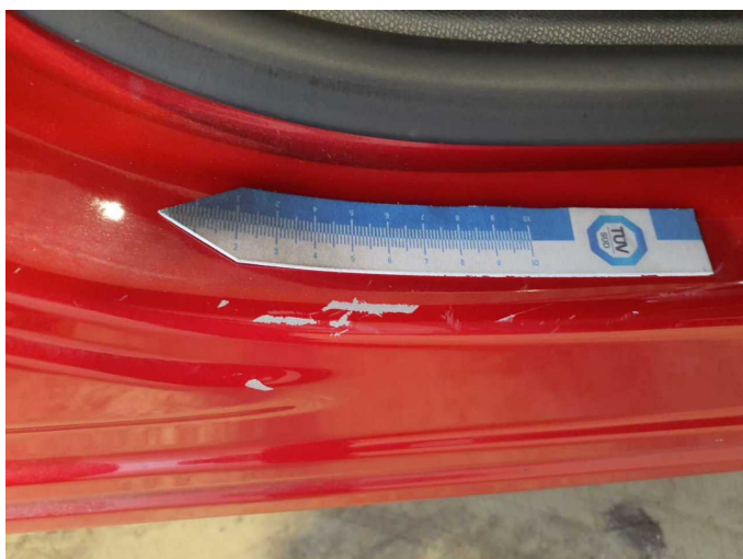
Damage 6: Sill - right side: Sill - Scratch(es) - Paint
