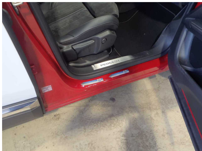
Damage 6: Sill - right side: Sill - Scratch(es) - Paint
