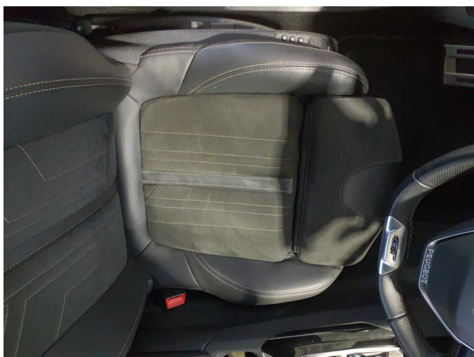
Damage 7: Seat - front: Seat cover - left side - Scratch(es) - Replace
