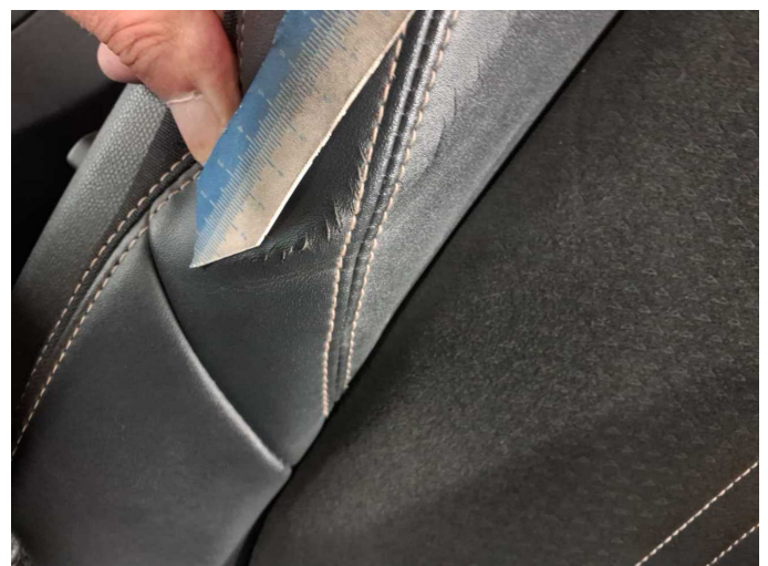
Damage 4: Seat - front: Seat cover - left side - Porous / cracked - Smart repair
