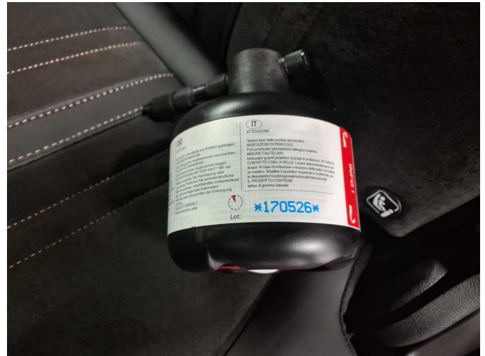
Damage 1: Equipment: Tirefit filler - Expired - Replace
