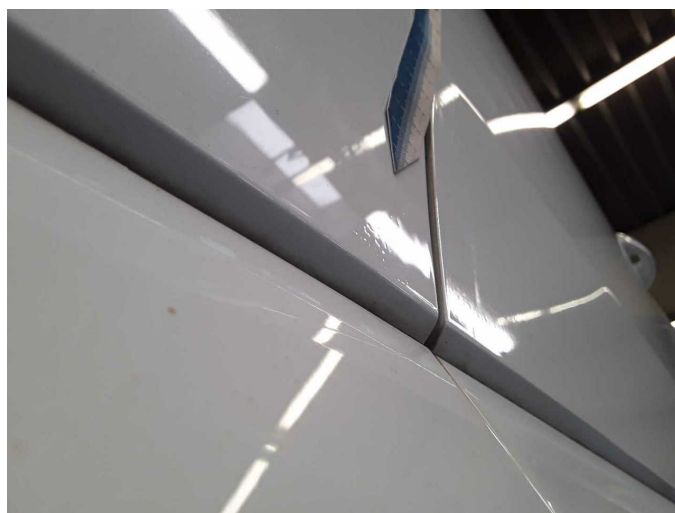
Damage 3: Door - front left side: Door (Orangenhaut + Silikon Einschlüsse) - Unprofessionally repaired - Paint
