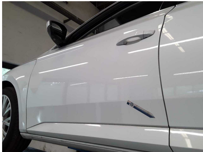
Damage 3: Door - front left side: Door (Orangenhaut + Silikon Einschlüsse) - Unprofessionally repaired - Paint
