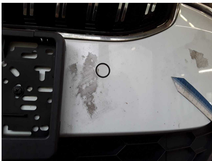
Damage 4: Front bumper: Front bumper (Lackabplatzer) - Paint defect - Paint
