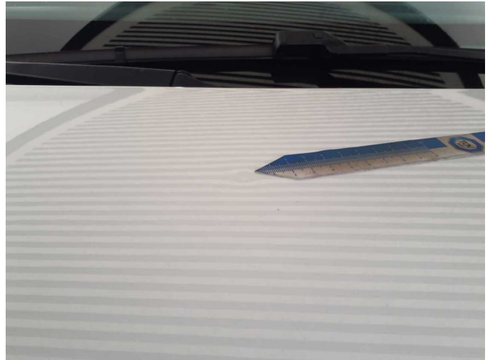
Damage 2: Bonnet: Bonnet - dent(s) - Smart repair
