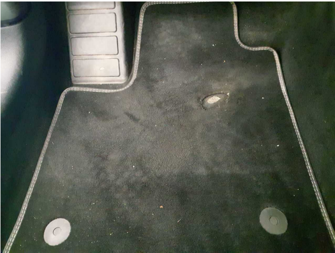
Damage 1: Trim / covers: Floor mats - Holes - Replace
