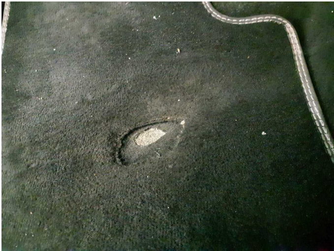
Damage 1: Trim / covers: Floor mats - Holes - Replace
