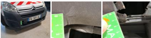
Bumper F, Broken, Repair and paint (complete)
