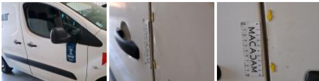
Door trim FR, Deformed / Strained, Replace
