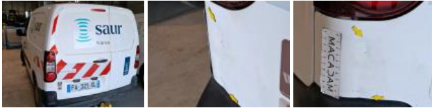
Bumper R, Deformed / Strained, Replace
