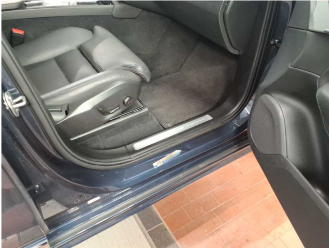
Damage 1: Sill - right side: Sill - dent(s) - Smart repair
