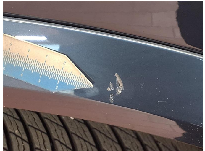
Damage 2: Mudguard - left side: Wheel well extension - Scratched - Smart repair
