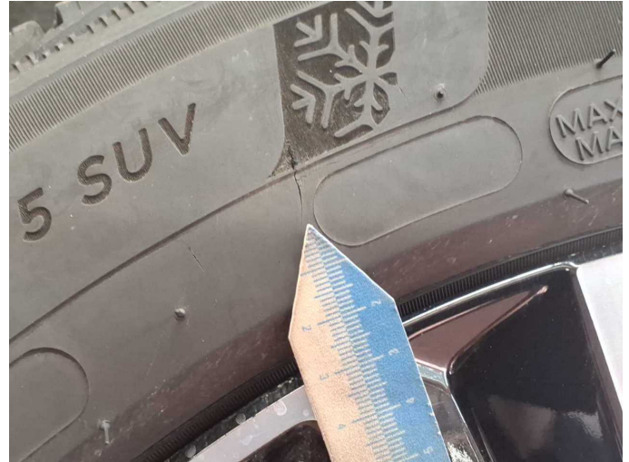
Damage 4: Wheel / tyres: Tyre - rear left side - Broken / torn - Replace
