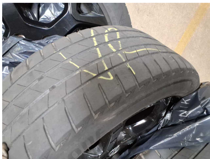
Damage 6: 2nd wheel set: 1 tyre (Flanke) - Damaged - Replace
