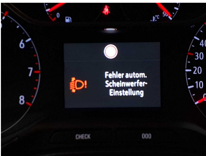
Damage 4: Electrical system: Lighting system - Functional / admissibility - Perform diagnosis
