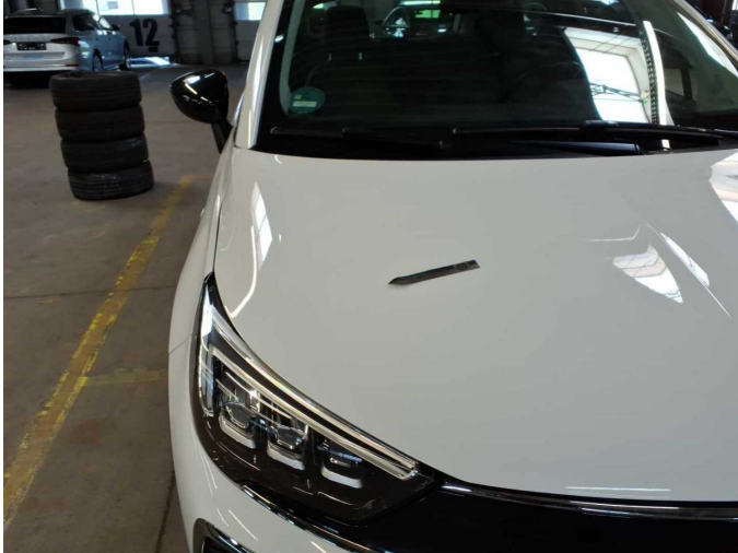
Damage 2: Bonnet: Bonnet - dent(s) - Smooth repair work
