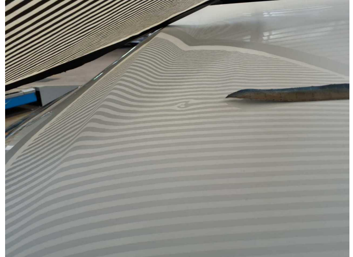
Damage 2: Bonnet: Bonnet - dent(s) - Smooth repair work
