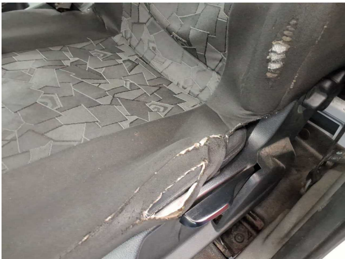
Damage 1: Seat - front: Protective Cover - left side - Damaged - Replace
