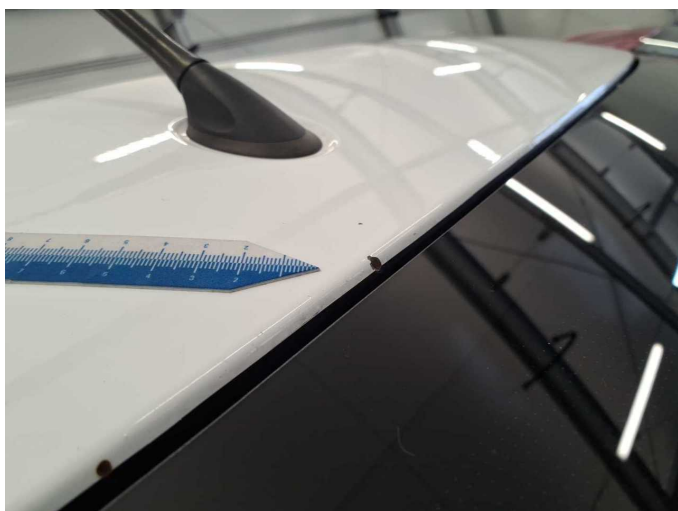
Damage 4: Roof: Roof (Dachkante) - Corrosion - Repair and paint
