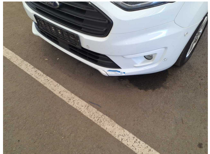
Damage 3: Front bumper: Front bumper (inkl. Parksensor) - Broken / torn - Replace
