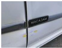
Sliding door R, Dent(s) and scratch(es), Repair and paint (complete)
