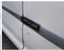
Sliding door R, Dent(s) and scratch(es), Repair and paint (complete)
