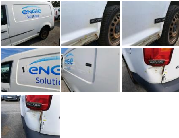
Door FL, Dent(s), Repair and paint (complete)
