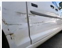
Sliding door R, Dent(s) and scratch(es), Repair and paint (complete)
