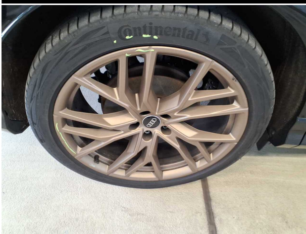
Damage #7: Wheel / tyres: Alloy rim - rear right side - Scratched - Loss in value
