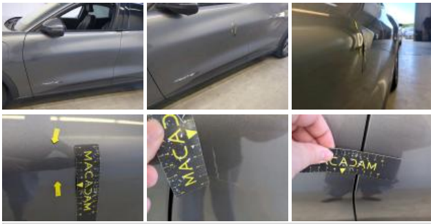
Door RL, Scratch(es), Repair and paint (complete)
