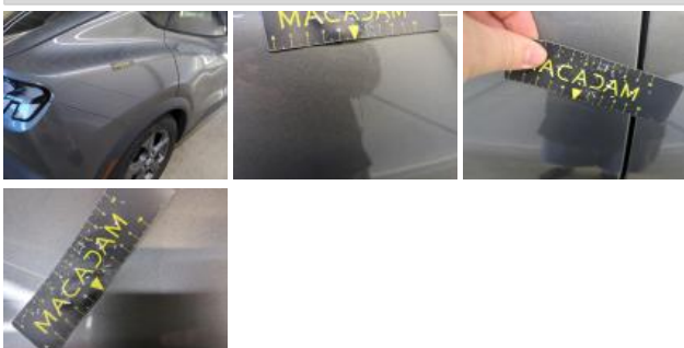
Door RR, Dent(s), Repair and paint (complete)
