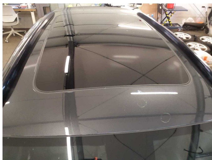
Damage 4: Roof: Roof (inkl. Holm links & rechts) - dent(s) - Smooth repair work
