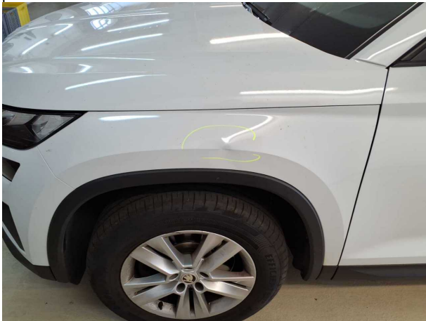
Damage #7: Mudguard - left side: Mudguard - left side - Dent / paintcoat damage - Replace
