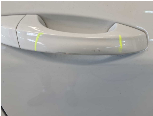
Damage #4: Door - front right side: Door handle - outside - Scratched - Smart repair
