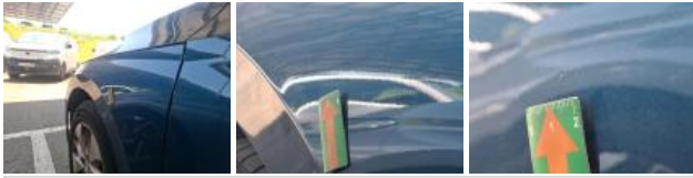
Door RL, Bad repair, Paint
