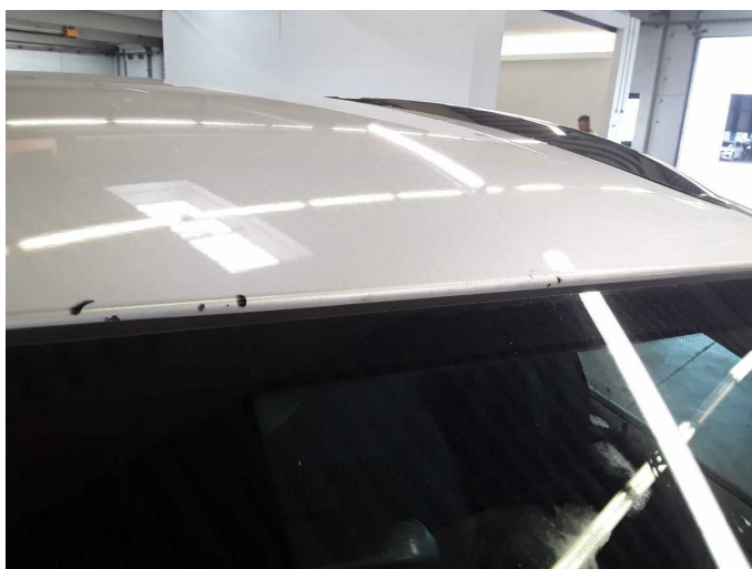
Damage 7: Roof: Roof - Stone chips - Paint
