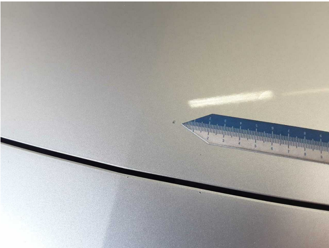
Damage 1: Bonnet: Bonnet - Stone chips - Smart repair
