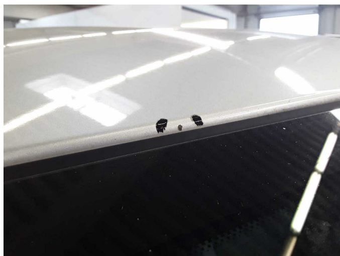
Damage 7: Roof: Roof - Stone chips - Paint
