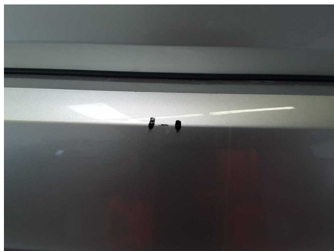
Damage 3: Rear bumper: Rear bumper - Scratch(es) - Paint
