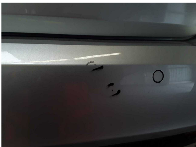
Damage 3: Rear bumper: Rear bumper - Scratch(es) - Paint
